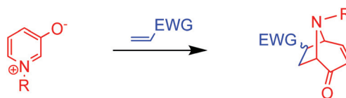
Scheme 4 3,2-Dipolarcycloaddition of 3-hydroxypyridinium betaines with electron poor ene.
